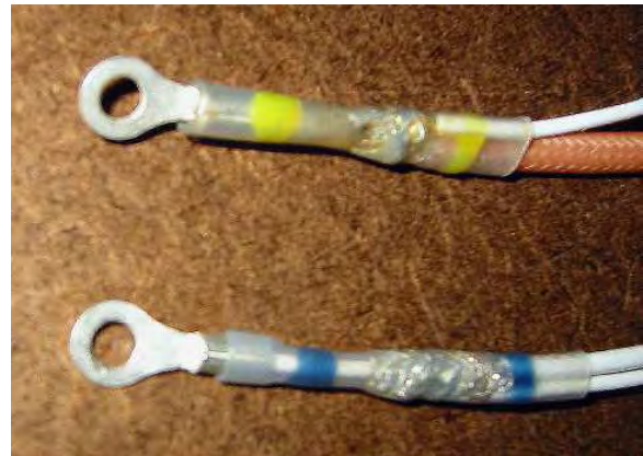
Magneto ring terminal connections soldered-heat-shrink with the shielded ground pigtail.
