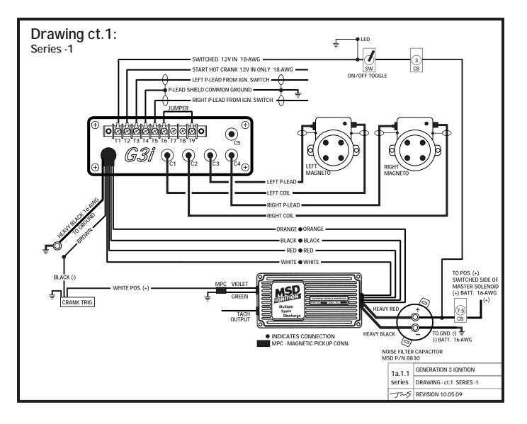
Crankshaft Trigger Signal Left Magneto Lag – Retard Impulse Coupler Left Magneto Normal Contacts are Trigger Source on Starting Bridge (T6 -T9) G3i Brown lead to Black (-) lead on Crank Trigger White (+) on Crank Trigger to Violet (+) on MSD amplifier Magnetic Pickup Connector Bare lead on Crank Trigger connector to common ground (-) Green lead on MSD amplifier Magnetic Pickup connector to common ground (-)
