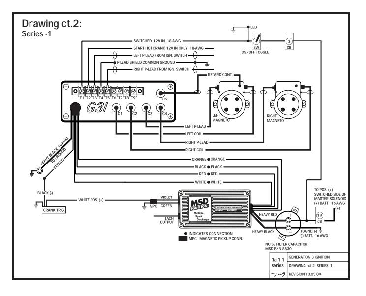
ODrawing ct.2: Crankshaft Trigger Signal Left Magneto Retard Contacts are Trigger Source on Starting Bridge (T6-T7) Retard Contact P-Lead to BNC (C5) G3i Brown lead to Black (-) lead on Crank Trigger White (+) on Crank Trigger to Violet (+) on MSD amplifier Magnetic Pickup Connector Bare lead on Crank Trigger to common ground (-) Green lead on MSD amplifier Magnetic Pickup connector to common ground (-)
